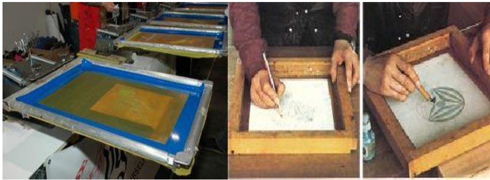
Figure No. (8-9) shows the steps for making a silk screen
